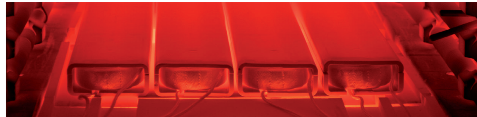
Burn-in test of the sensor coils in the purpose-designed furnace by EMG
